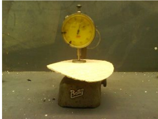
dial indicator measuring thickness of ecoYoga material 2007
